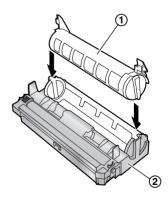
8 Firmly press down the toner cartridge to snap into position.
